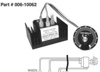
The Power Control Module offers infinitely variable phase control when used with resistive loads up to 25 amps. The solid state circuitry provides modified transient suppression, exceptional stability and life. An external potentiometer/switch (dial plate and knob included) is used to control output voltage. A trimming potentiometer is mounted on top of the module to adjust turn on voltage level. This device should be installed in a circuit fused at 120% rated load or 30 amps maximum.
